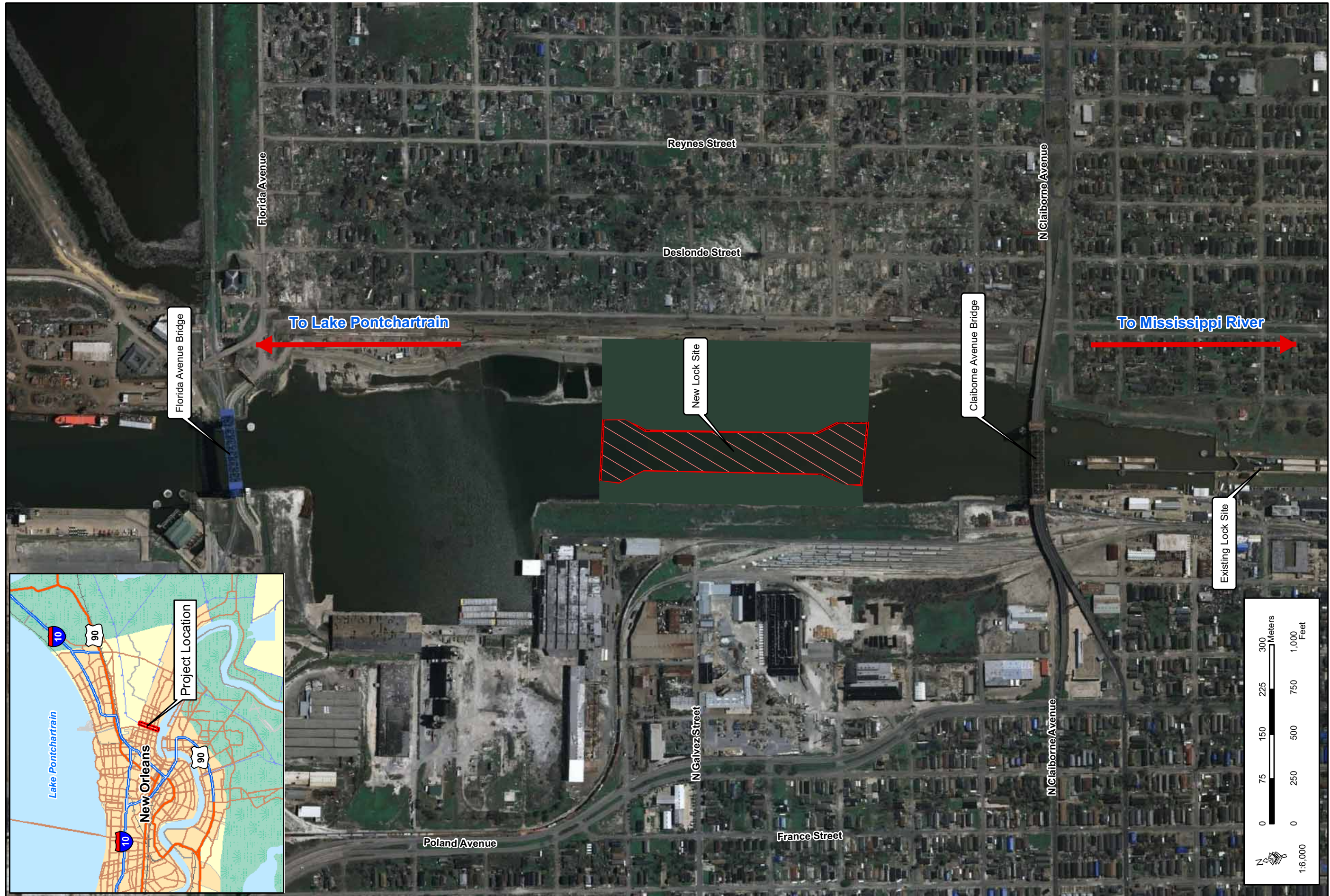
Figure 4-3: Footprint of Proposed Lock (110 feet wide; 1,200 feet long; and 36 feet deep at its location as shown in the FIP vs CIP Letter Report exhibits)
